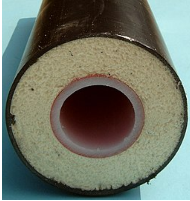
Figure 3.1: The thermal insulation of a pipe (photo by Sönke Kraft aka Arnulf zu Linden on commons.wikimedia.org).
